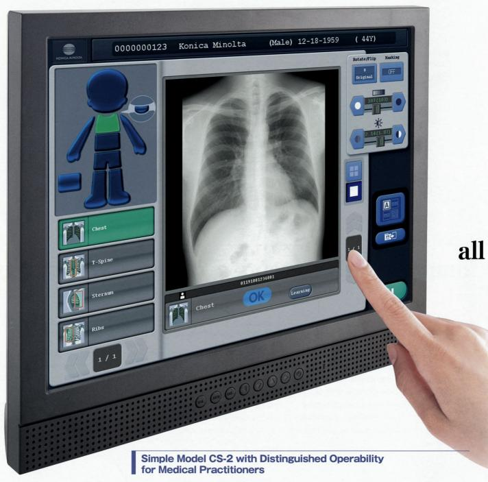
This Regius console features a user-friendly screen layout with intuitive, easy operability and a body shaped icon. The image-processing functions provide optimal images by body part. In addition, the unit stores information on adjusted image density and contrast, automatically customizing the finished images to suit the customer's needs.
